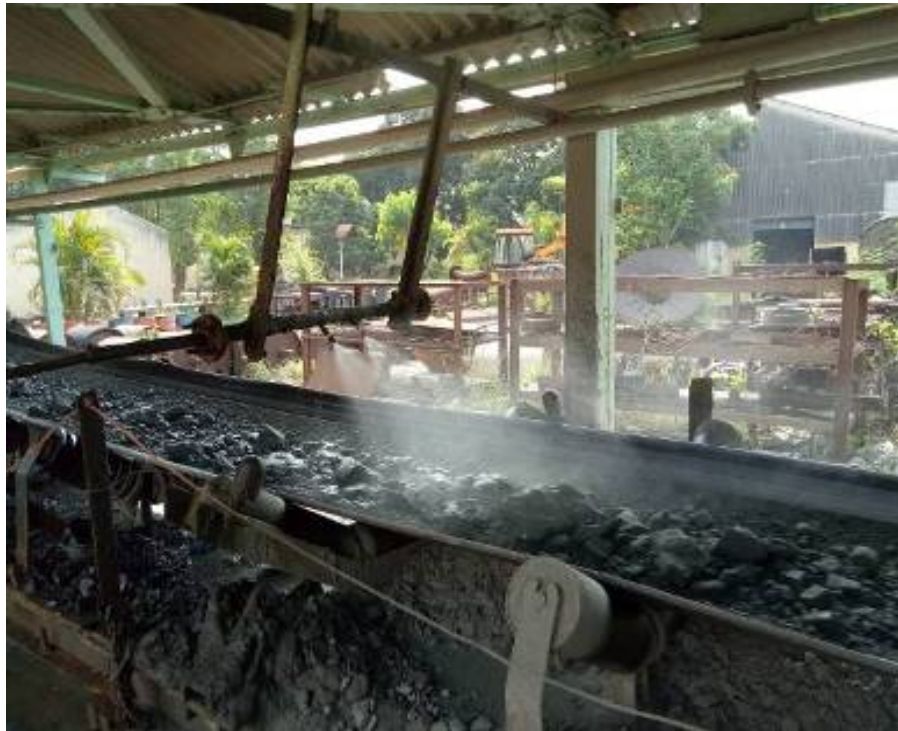
Photograph of water sprinklers at ore handling area
